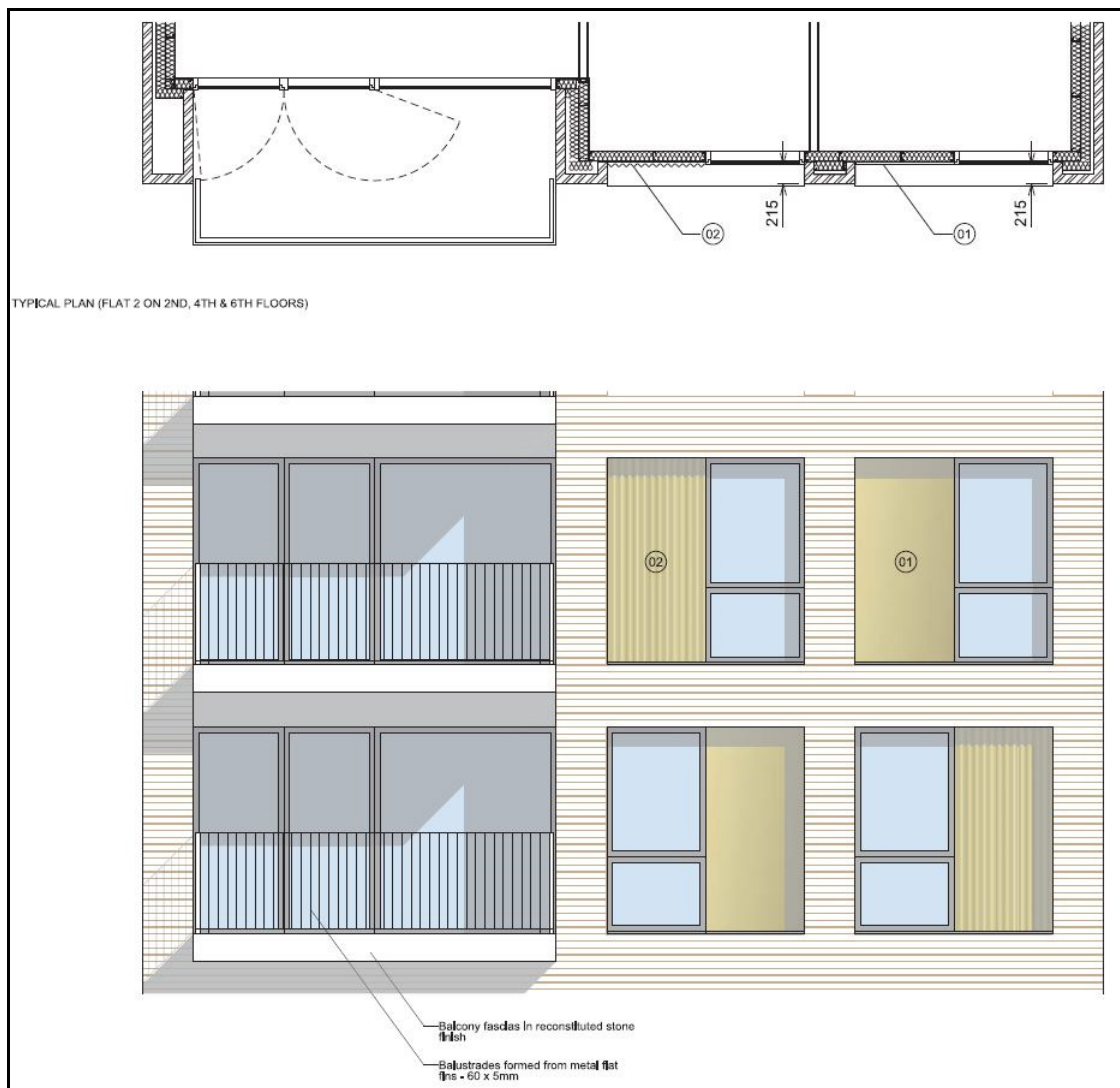
Figure 9: A typical bay study, showing the depth of reveals and the details of the junction between the balcony decks and the elevations.
